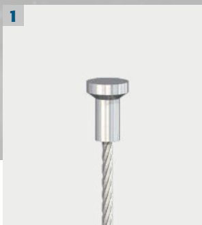
1 T-sleeve 02 Head Ø 6.0 mm Shaft Ø 3.5 mm Length 8.5 mm
